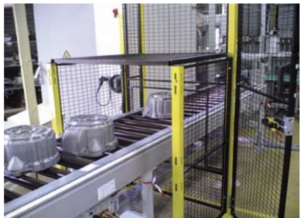
FlexiGuard as protection around a tunnel to prevent operators to get their arms through the conveyor. This solution is frequently asked for within the automotive industry.
