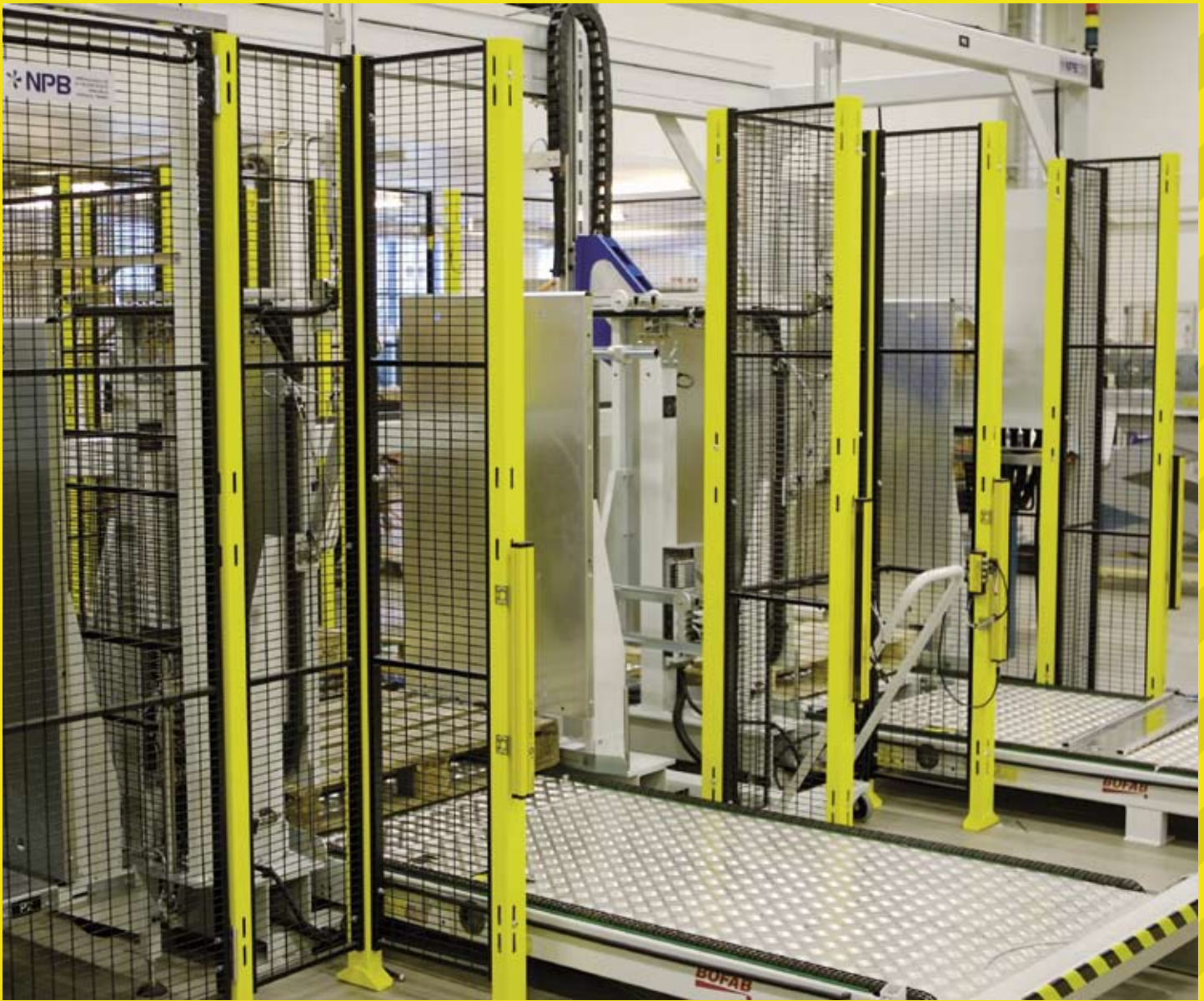
▲ MasterGuard around a fully automated palletiser for bagged or wrapped ends produced at NPB Automation AB in Sweden.
