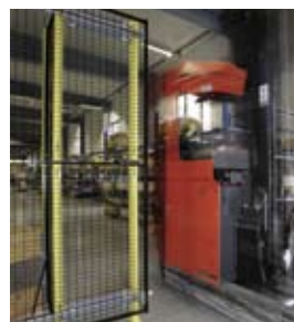
Sliding door without rail: Ideal where material refilling, truck driving and crane loading are usual.
