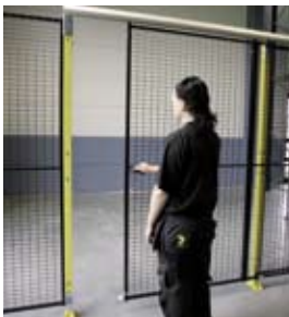
Single sliding door: Good option when there is not enough space to open a hinge door.
